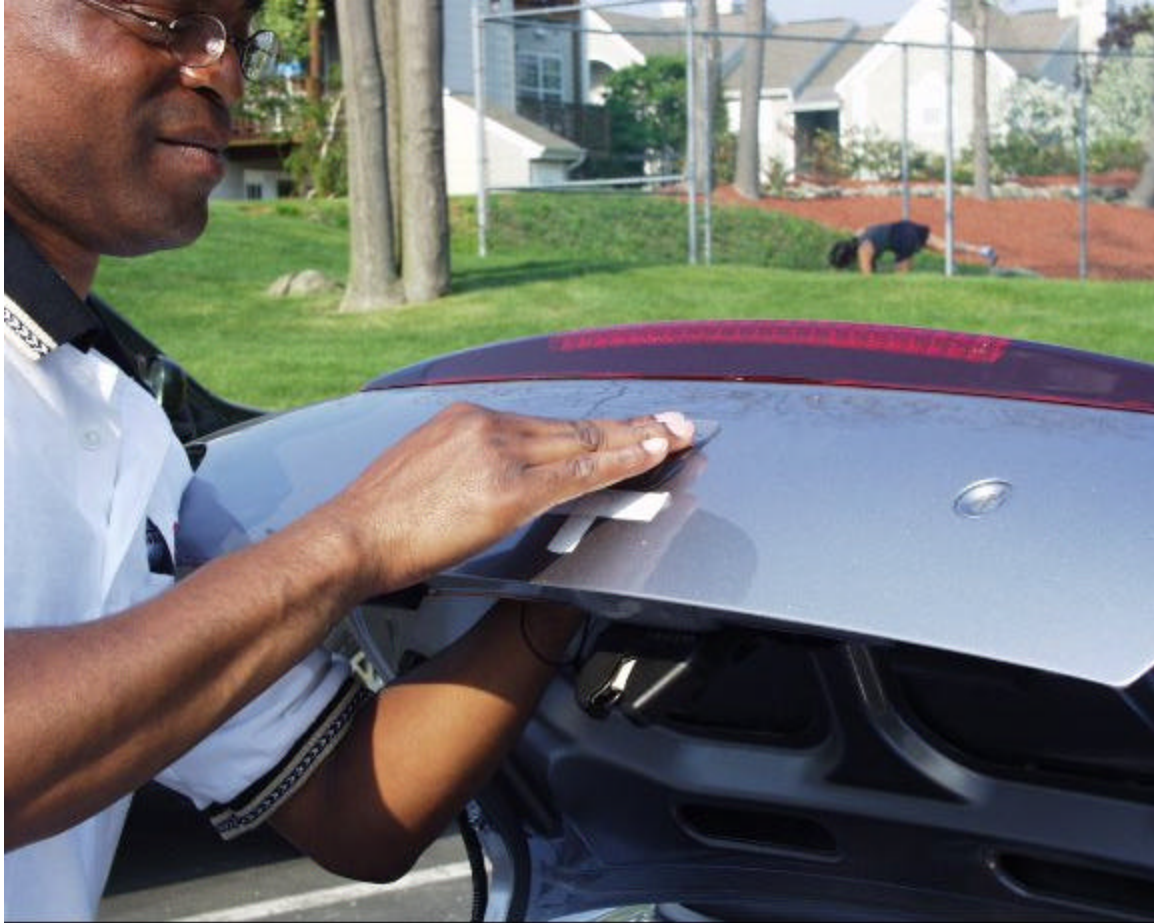
Figure 20 Rear Badge Installation
